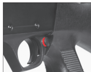
"Safety" shown in the off safe position.
