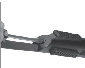
Carefully remove the forearm attachment nut with a screwdriver.
