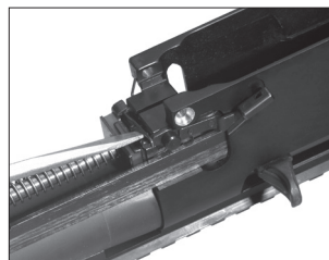
Release the bolt lock spring.
