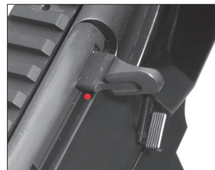
Verify the bolt is fully forward.
