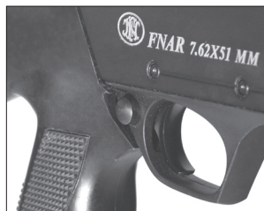
"Safety" shown in the on safe position.
