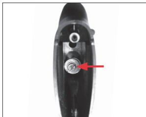
Carefully remove the screw that secures the buttstock.
